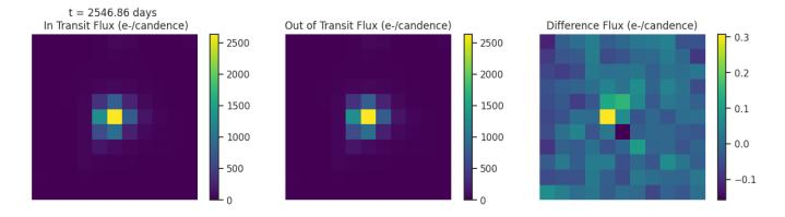
Fig 6. Difference images for target TIC 171600318 for each transit like event. Left: mean in-transit flux(left). Middle: mean out-of-transit flux. Right: difference between the mean out-of-transit and mean in-transit flux. Ensure that the change in brightness occurs on target.
