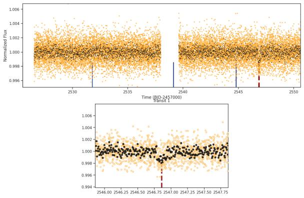
Fig 1. Full lightcurve for target TIC 171600318. The solid blue lines at the bottom of the figure indicated the times of the reaction wheel momentum dumps and the dashed black line(s) show the time(s) of the marked transit event(s). Momentum dumps occur around every 2 to 2.5 days and typically last around half an hour.
